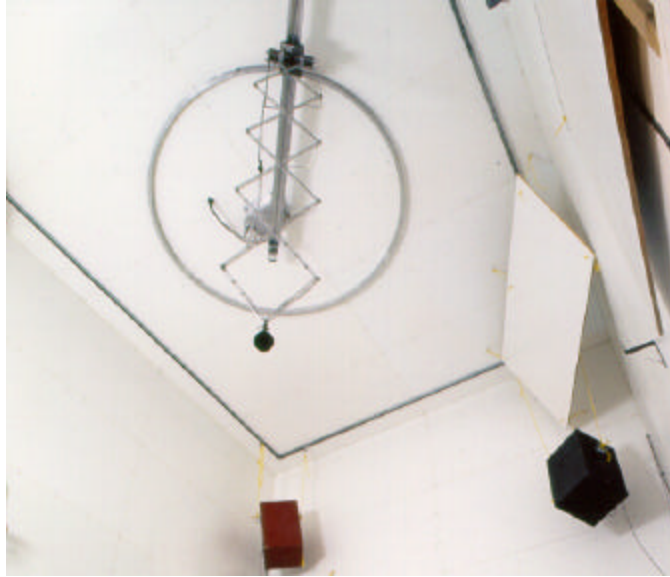
Figure 4: Automated system for moving the microphone in each room. Two of the four loudspeakers used in each room are visible in the picture.
